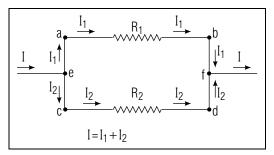
Fig. B-2: Resistors connected in parallel.
