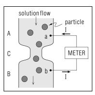
Fig. F-1: Electric measurement of number and sizes of particles in a solution.
