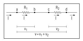
Fig. B-1: Resistors connected in series.
