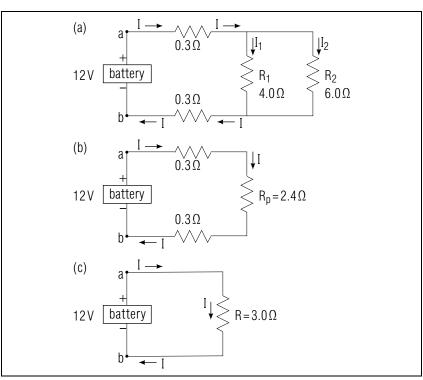
Fig. C-1: Circuit representing a battery connected by wires to two lamps. (a) Original circuit. (b), (c) Circuits equivalent to the original circuit.
