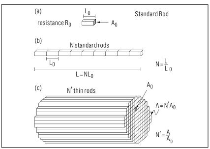
Fig. D-1: Combining small standard rods to make other rods.
