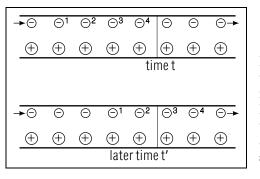
Fig. A-2: Motion of electrons through a metal wire with no net charge. The diagram illustrates very schematically the positions of the electrons and stationary ions at two slightly different times.
