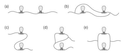
Which of the preceding diagrams show the bulbs connected in series and which show the bulbs connected in parallel?
