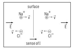
Fig. A-4: External electric field  $\vec{E}$  causing motion of Na<sup>+</sup> and Cl<sup>-</sup> ions in a solution of sodium chloride.
