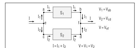
Fig. E-3: Two-terminal systems  $S_1$  and  $S_2$  connected in parallel.
