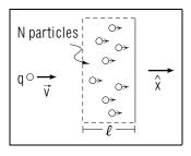
Fig. B-2: Moving charged particles passing through a surface.
