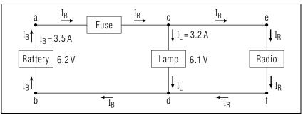
Fig. E-1: Circuit consisting of a storage battery connected to a lamp and a radio.
