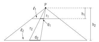
The preceding drawing shows two lines  $(\ell_1 \text{ and } \ell_2)$  each with the same charge per unit length  $\lambda$ . Line  $\ell_2$  is 3 times as far from P as line  $\ell_1$
