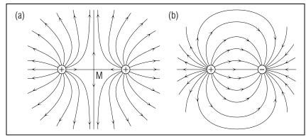
Fig. C-3: Electric field lines due to two particles having charges of the same magnitude. (a) Both charges positive. (b) Charges of opposite signs.
