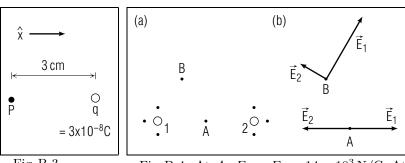
Fig. B-3. Fig. B-4: At A:  $E_1 = E_2 = 14 \times 10^3 \text{ N/C}$ . At B:  $E_1 = 12 \times 10^3 \text{ N/C}$ ,  $E_2 = 5 \times 10^3 \text{ N/C}$ .
