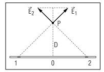
Fig. E-2: Edge-on view of a uniformly charged plane and of the electric fields produced at P by charges on two symmetrically located equal small portions of the plane.
