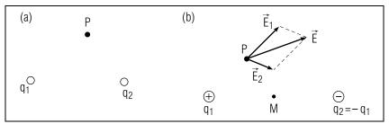
Fig. B-2: Electric field due to two charged particles. (a) Point *P* near two particles. (b) Electric field at points near a dipole.
