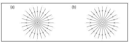
Fig. C-2: Electric field lines due to a single charged particle. (a) Positively charged particle. (b) Negatively charged particle.
