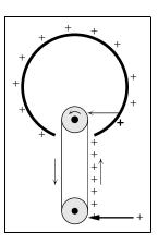
Fig. D-1: Schematic diagram of a Van de Graaf generator.
