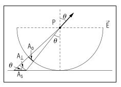
Fig. H-3: Edge-on view of a uniformly charged plane, showing the electric filed produced at P by the charge on a small square of this plane.
