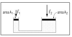
Fig. D-3: A hydraulic press
