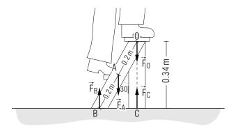
and we wish to find the magnitudes of the upward forces  $\vec{F}_B$  and  $\vec{F}_C$  exerted on the stepladder by the floor at the points B and C. The remaining external force on the stepladder, the gravitational force, is negligible.
