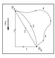
Fig. A-1: Work done on a particle along various paths between two points. (The arrow indicates the direction of a constant force  $\vec{F}$ .)
