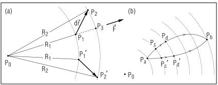
Fig. C-1: Work done on a particle by a central force due to a particle fixed at  $P_0$ . (a) Small displacement. (b) Displacements along two different paths between the same points.
