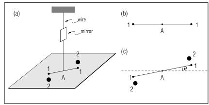
Fig. D-1: Cavendish experiment for the determination of G. (a) Perspective view of the experimental arrangement. (b) Top view of the lead spheres 1 originally at rest. (c) Top view of the lead spheres 1 finally at rest in the presence of the lead spheres 2.
