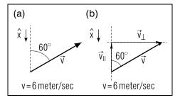
Fig. B-1: Components of a velocity. (a) Velocity  $\vec{v}$  of a jumping rabbit. (b) Component vectors of this velocity.
