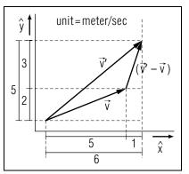
Fig. D-1: Subtraction of two vectors.
