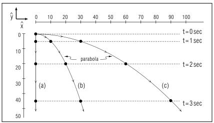
Fig. E-2: Path of a particle moving under the influence of gravity near the surface of the earth after being projected with a horizontal velocity  $\vec{v}_A$ . The dots indicate successive positions of the particle. (a)  $-\vec{v}_A = 0$  (b)  $\vec{v}_A = (10 \, \text{meter/sec})\hat{x}$  (c)  $\vec{v}_A = (30 \, \text{meter/sec})\hat{x}$ .
