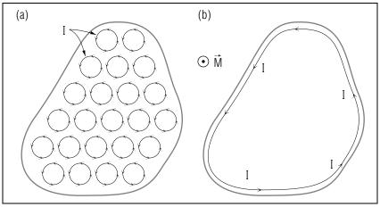
Fig. B-1: End-on view of a magnetized rod. (a) Atomic current loops. (b) Equivalent current around the periphery of the rod.
